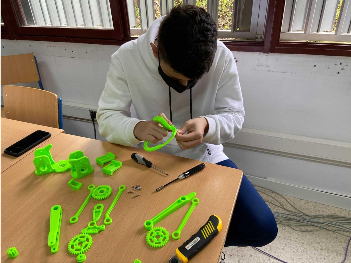
As specified in another unit, one of the steps we have done to build our rover is to create a robotic arm. This arm was built with the aim of being able to adapt and transform it for our system.
