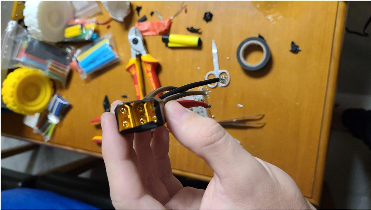
For the connection of the batteries we have used XT60 connectors. They are profusely used in modeling.
