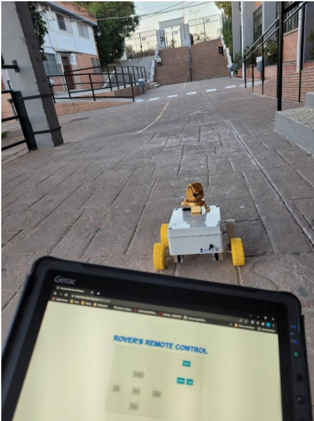
The objective of our system is to implement a websocket client in such a way that it listens at all times to the server implemented in the cloud. Every time the server detects that the user makes a move, it quickly sends it in GCode format to the client located on the rover.
