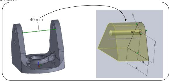
**Fourth step**: Find and add dimensions from the detector to the new design part. Students have to visualize the model in 3 dimensions to transfer the dimensions on the good plane. The real part of the detector helps students to do that.
