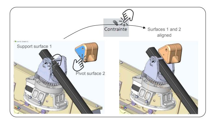
Same operation for the axis of the support and the axis of the pivot :
