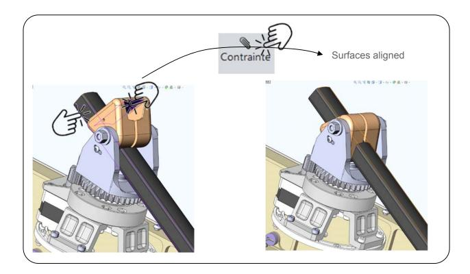
**Last step**: The last link is between the adjusting screw and the pivot. Some other links can be added, for example, the distance between the end of the detector and the pivot...
