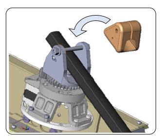
**First step**: The CAD function which allows to assemble 2 parts is based on selection of contact surfaces between the 2 parts to be assemble.
