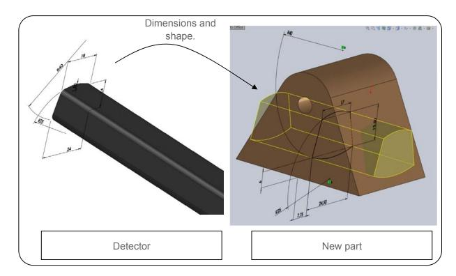
**Fifth step**: Add the technical function: adjusting the detector position. A drilling thread is added to adjust the detector position on the arm support. A slot must also be added to tighten the detector in position. There are many solutions to solve this technical function, students have to find one. The 3d print allows to try easily if the chosen solution is compliant.
