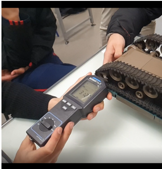
measurement of the rotation frequency of the driving wheel N = 250 \text{ r. min}^{-1}
